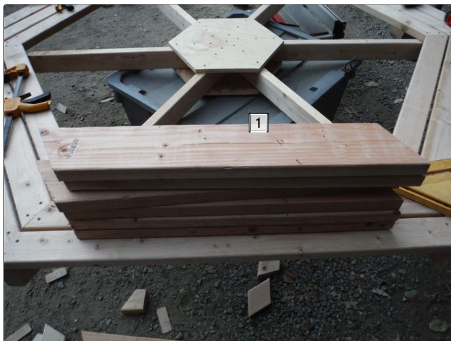
1. mark a line 20 1/2" from the bottom and parallel with the cut ends on each leg
